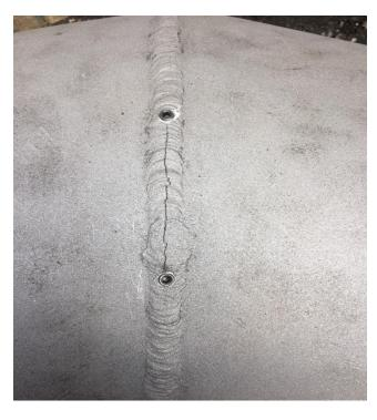
To make a full evaluation of the repair, a temporary wrapping, which had been placed around the pipe, was removed. The pipe was then cleaned and, the welded joints were grit blasted. On close inspection of the area around the escape it was revealed that there was a crack in the central welded joint.
